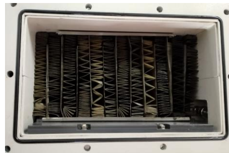
Collectors- After Filtration
