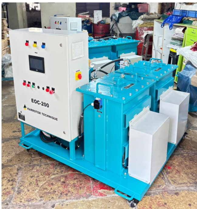
EOC-200 model with Online Particle Counter, touchscreen HMI, PLC
