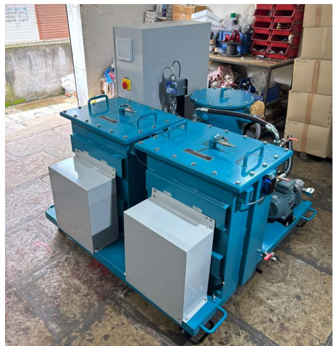
EOC-200 model with Online Particle Counter, touchscreen HMI, PLC
